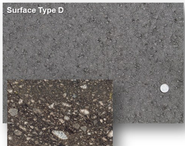
Figure 3.3. Surface texture comparison for surface course types B, C, and D. The inset photos show a cross-sectional view of each mix type. A US quarter is used as a scale reference.
